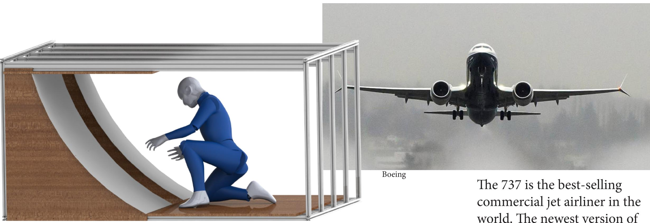
We designed and built a mock cargo bay in order to test our desgins and potential solutions and compare it to the current installation experience of the workers.
