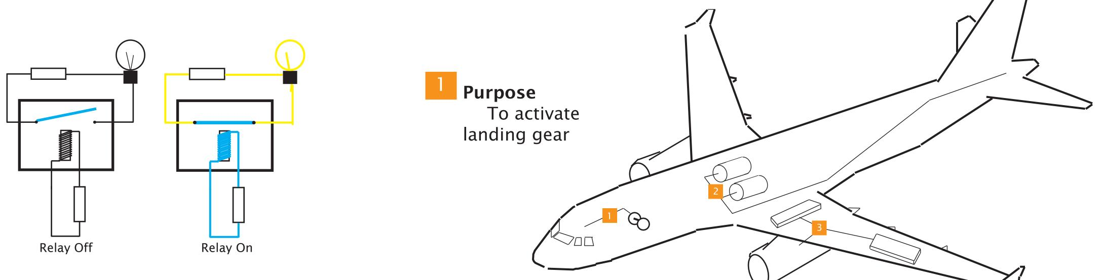
*Relays* are electrically activated switches that allow current to flow when turned on.
