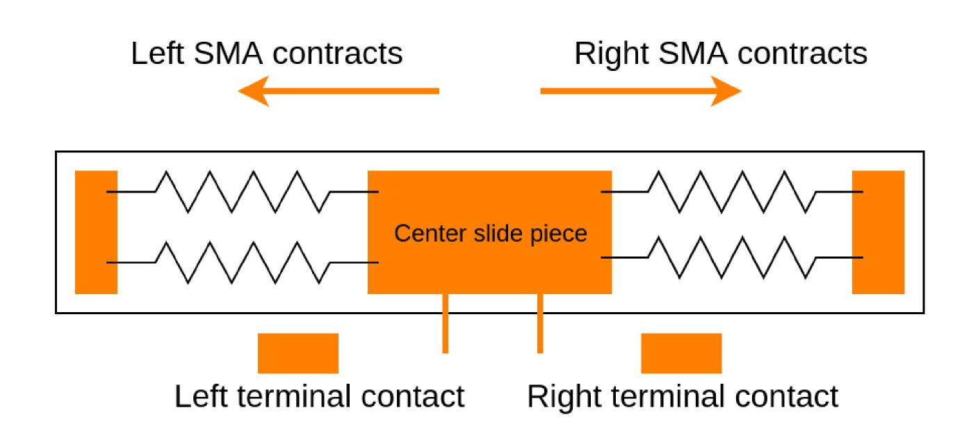
The actuator is made up of three portions, two sets of SMA's, a center slide piece and the electrical contacts. Each set of SMA's are powered independently to pull the center slide piece, by contraction, to its respective side.
