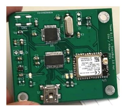
Our custom hardware is equipped with a suite of sensors, a power conversion unit, and all of the RF components necessary for communicating over a Zigbee network
