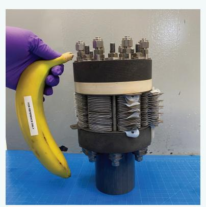
Static Vapor Feed Electrolyzers (SVFEs) have a simpler support system compared to traditional liquid feed electrolyzers. The cell stack (left) is where the electrolysis reaction occurs.
