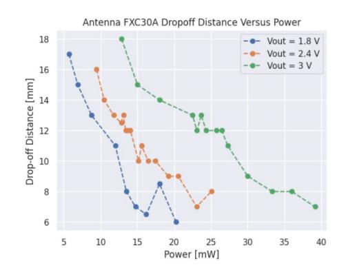
The graph to the left shows the change in drop-off distance depending on the system when using the 30 mm circular antenna. We found that many temperature sensors use between 0.5 and 5 mW of power.
