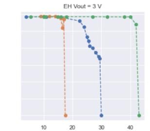
These graphs show the varying drop-off distances of three of the antennas we decided to test at 1.8, 2.4, and 3 V outputs. We find that at the 3 V output setting, the 30 mm circular antenna is able to transmit data at the furthest distance.
