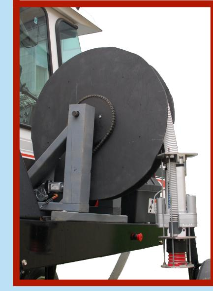
Magnets align and connect valve assemblies
