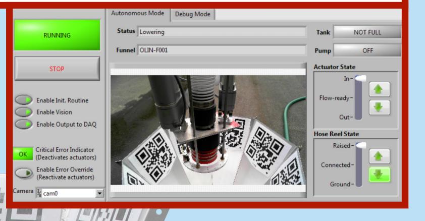
Funnel guides male valve into alignment with female valve
