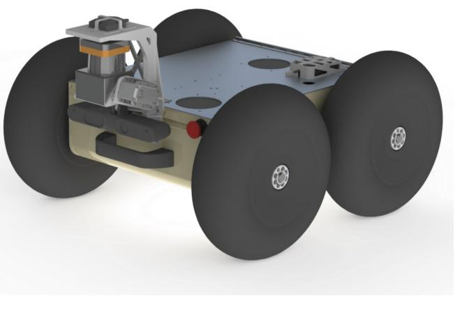
can drive over obstacles up to 4-5 inches and on slopes up to 40°. It can also drive on a wide variety of terrains including carpet, grass, gravel, and mud. The robot can withstand falls and bumps associated with a testing environment and is designed to protect sensors from reasonably foreseeable incidences.
