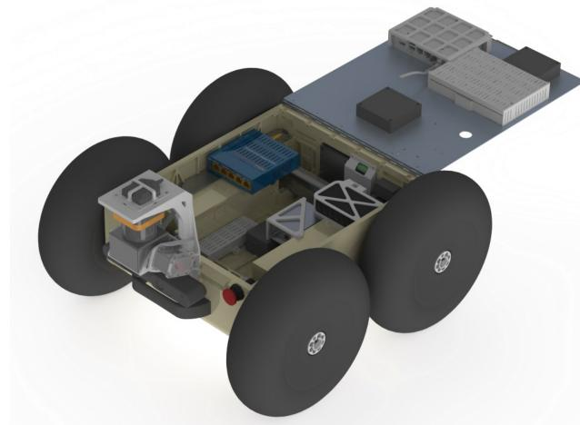
The electrical system uses two 22.2V batteries to provide power to two onboard PCs as well as their I/O interfaces, an Arduino and powered USB hub. It also powers the motors, motor controller, and a set of fans to keep all electrical components COO.
