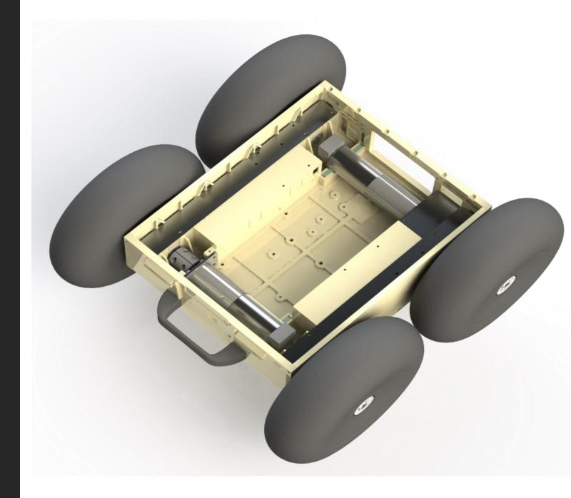
chassis is The constructed from fiberglass, ероху coated FDM ABS. The drivetrain is wheeled simple skid steering. The vehicle can travel at speeds up to 2.3 m/ The vehicle
