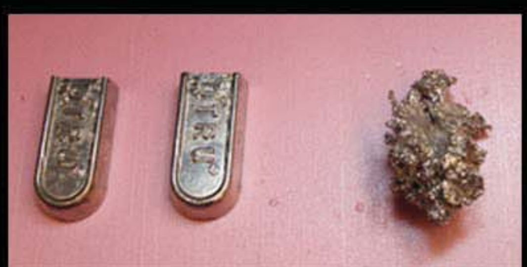
Modular External Ballast Filled with Tin-Bismuth Alloy, Fine Tuning Through Steel Ball Bearings
