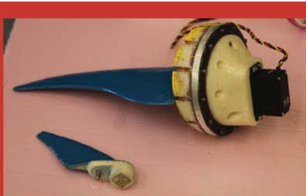
Pectoral Fin Actuated by Servo and Pneumatic Vane Motor
