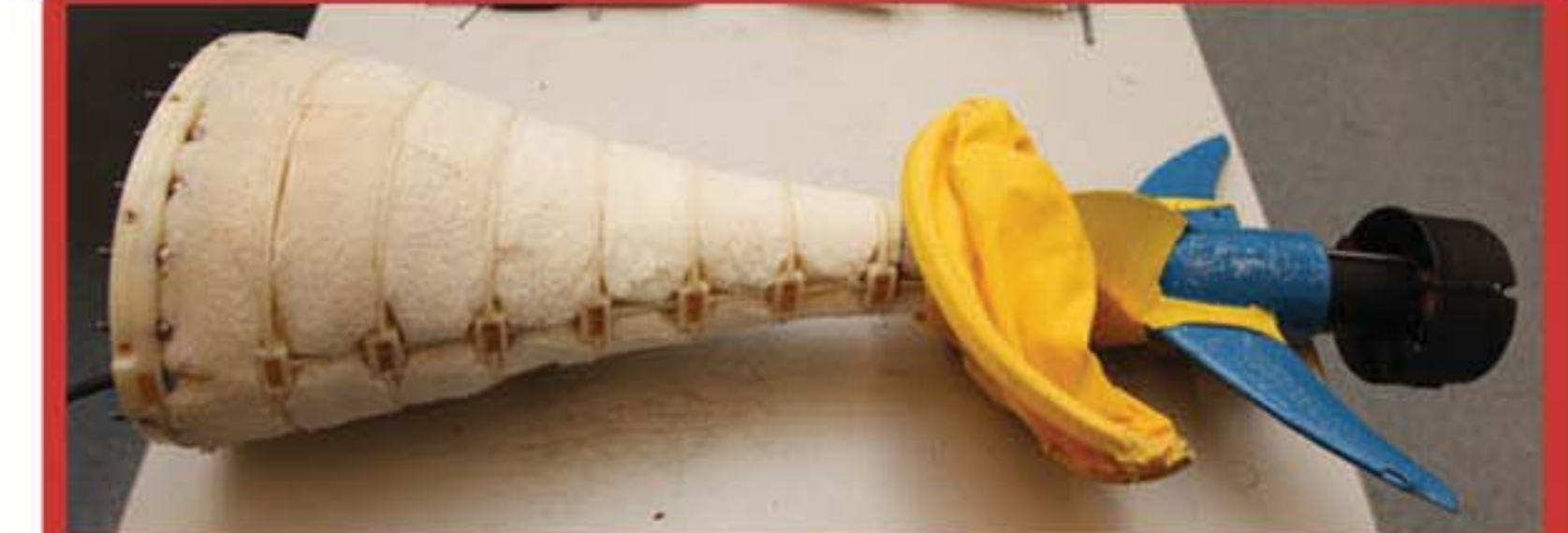
ABS Plastic Skin Support Structure with Flexible Polyurethane Foam Covered with Lycra Skin
