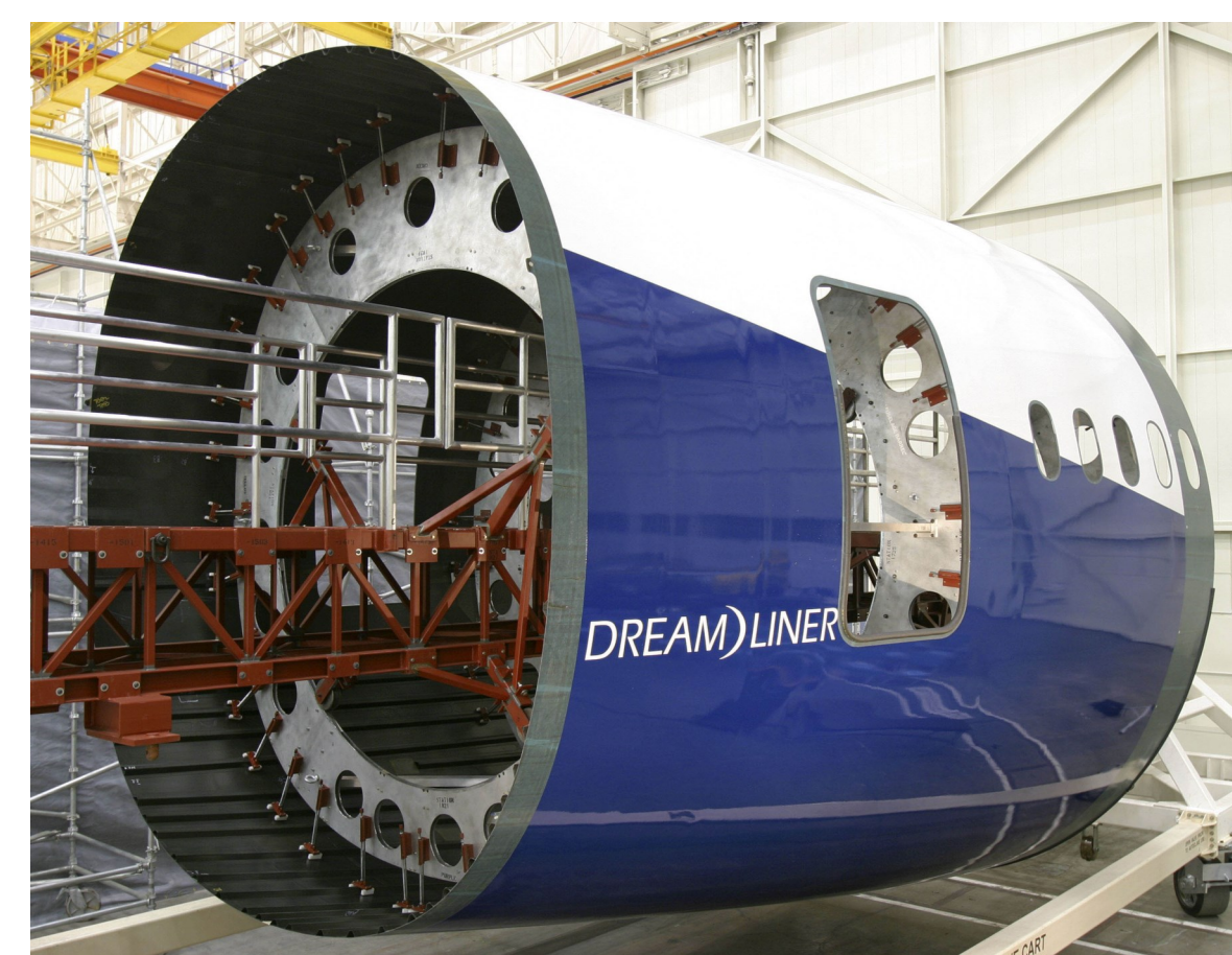
Current use of carbon fiber in the Boeing 787 Dreamliner fuselage [3]
