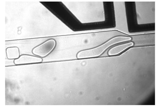
Two droplets prior to merging; 40VDC applied across the electrodes.
