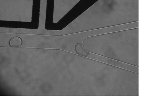
Droplets being steered to the upper path; 200VDC applied across the electrodes.
