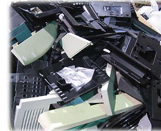
After dismantling, plastic components such as these are left behind. Plastic piles like these contain several different types of plastics, but most notably HIPS, ABS, and PPE.
