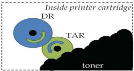
Toner is collected from the toner adder roller (TAR) and transferred to the developer roller (DR) through frictional triboelectric charging and electrical biasing from the rollers. The remaining steps in the laser-printing process depend on the charge obtained by the toner in this initial phase.
