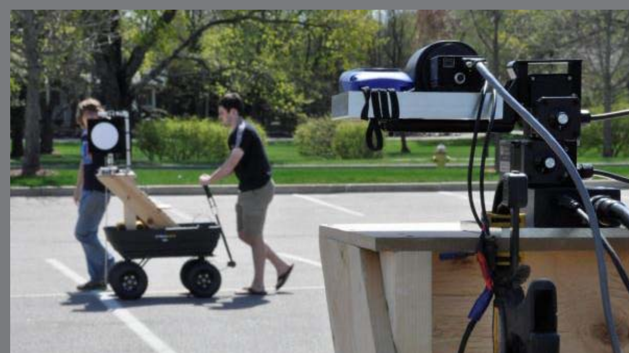
Here the lead system is being pulled between two points on the circle. The follower system tries to keep track of target as it moves back and forth.
