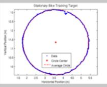
Figure 1: This image shows a circle we traced out with the target while keeping the bike stationary. Overall, it is very circular (especially compared to the red outline) with small deviations that are mainly caused by the difficulty in keeping the target perfectly aligned while walking about the circle. This test indicates that we can achieve good precision with our system.
