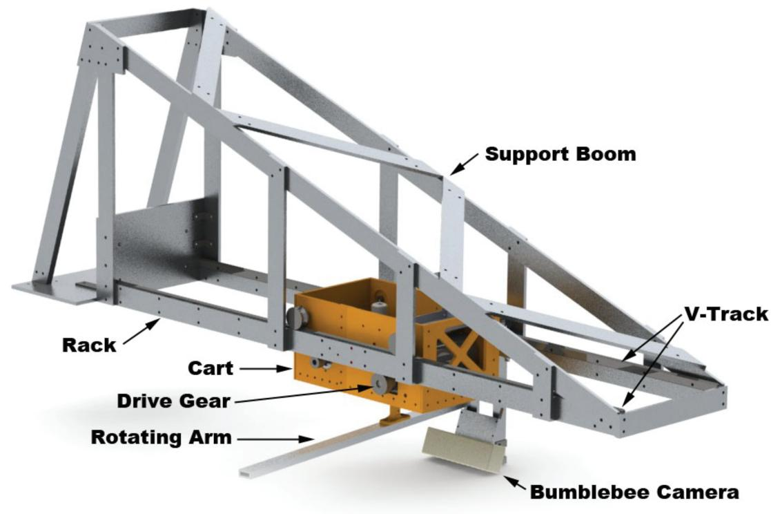
The system uses a cart with a rotating arm that rides along a boom to position a laser pointer over the center of a hole. PID controls programmed on an Arduino Uno to actuate the cart and arm motors, moving the laser pointer over the detected hole center. Rotary encoders continuously update the cart and arm positions. The motors, encoders, and arduino are housed inside the cart.
