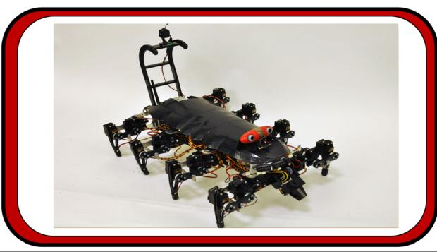
FINAL DEMO: The robot will search the environment for the target: a red circle. Once found, it will walk in a straight line towards the target. If an obstacle is detected in its path, the robot will follow a designated sidestepping response to walk around the obstacle. Once the obstacle is cleared, the robot will search for the circle-target once again and continue walking towards it. The robot will stop once it reaches the target.
