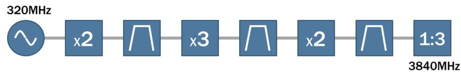
Currently the generation of low phase noise oscillators in the microwave frequencies is done by using multipliers to convert an extremely stable but low frequency oscillator up to the desire frequencies. Though this method does produce low phase noise microwave frequency oscillators, there are drawbacks. Each multiplier and necessary band-pass filter both attenuates and adds more noise to system. This means there high frequency systems are usually extremely large and inefficient.
