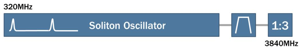
The soliton oscillator system would get rid of many of the multiplier and band-pass filters. Since solitons have many harmonics, all that is needed to get microwave frequencies is a band-pass filter at the desired frequency.
