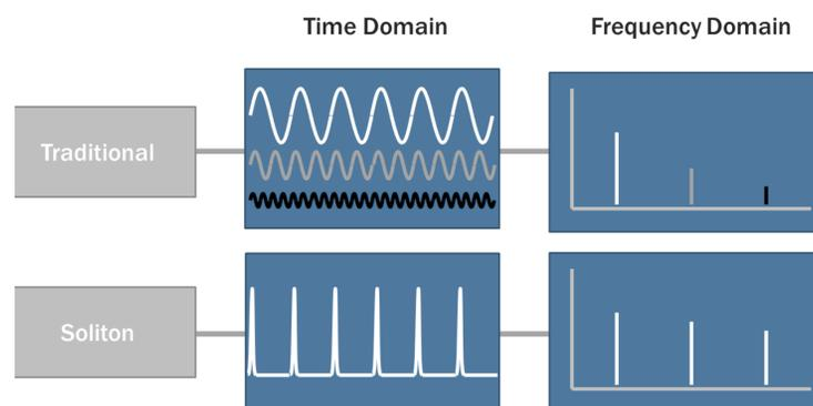
The diagram to the left shows the differences between the traditional method to create high frequency oscillations and the new soliton oscillation method.
