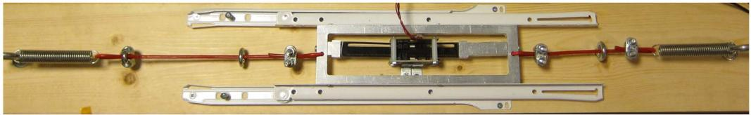
Velocity sensors help to differentiate between a slow, small linear change from thermal expansion and a fast linear change from an emergency pull
